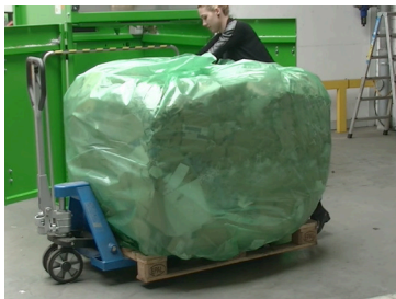
Bag on pallet is removed by pallet jack
